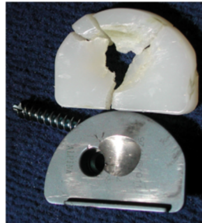
Radiological wear of PE insert 7%
